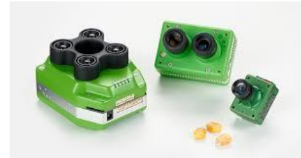
Lightsensor, multispec (R, G, RE, NIR; 1280*960), different cameras and bands
