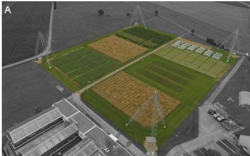
Rope suspended Field phenotyping platform (FIP) Kirchgessner et al 2016, FPB
