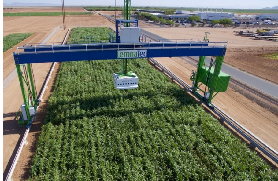
Field Scanalyzer, an automatic sensor-to-plant system in which a camera can be mounted on the probe head.
