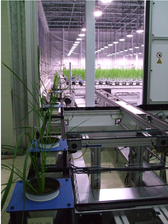
Greenhouse Scanalyzer, an automatic plant-to-sensor system in which hyperspectral cameras can be mounted into measurement cabins.
