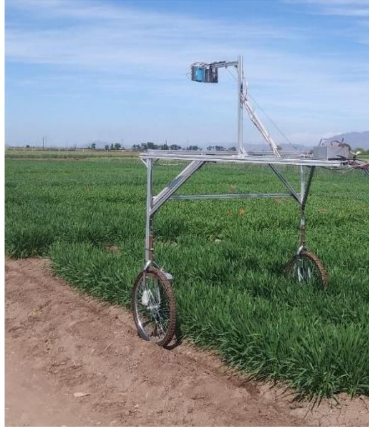
Terrestrial vehicle for integrated measurements of different sensors:
