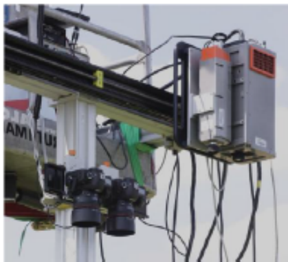
SLR-cameras on a sliding bar + hyperspectral imaging
