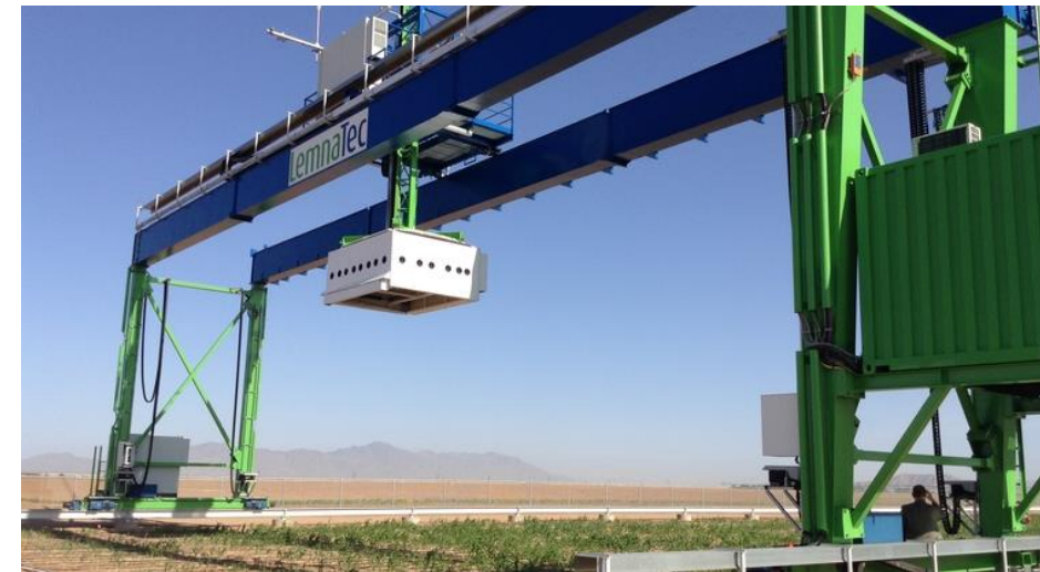
The world's largest robotic field scanner (white steel box) is mounted on a 30-ton steel gantry moving along 200-meter steel rails over 1.5 acres of energy sorghum at the Maricopa Agricultural Center. (Photo: Susan McGinley)
